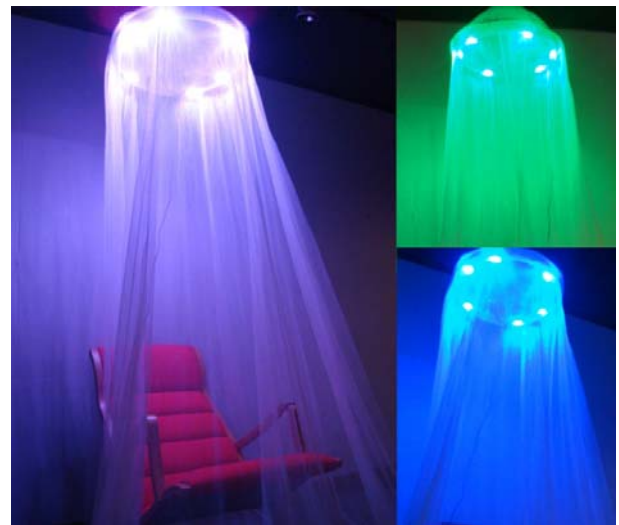
Fig.4. LED lights hanging from the ceiling over the chair can illuminate an arbitrary color to the veil surrounding the chair
