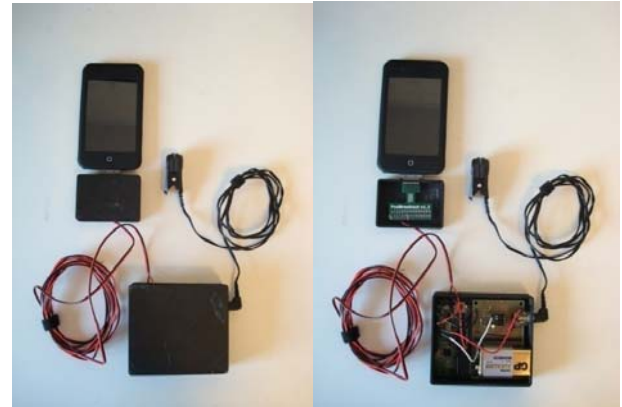
Fig.3. An iPodTouch with a pulse sensor and an amplifying circuit.
