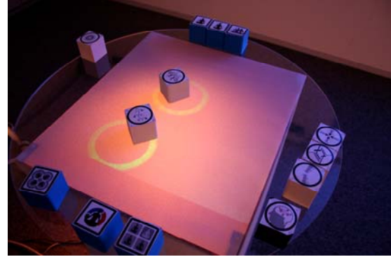
Figure4. Tangible Objects on the table top. When user places material objects, the green circle animation appears under the object.
