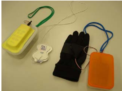
Figure6. Glove with embedded sensor (right) and low-frequency pad (left)
